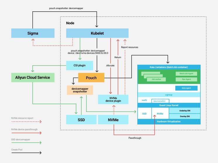
Figure 6: Kata Containers Storage Architecture Diagram
