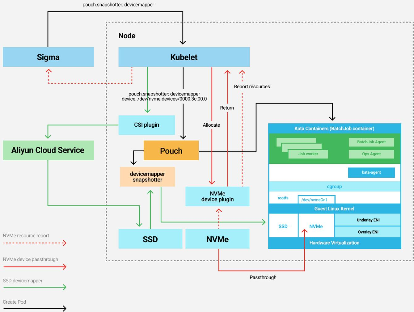
Figure 6: Kata Containers Storage Architecture Diagram
